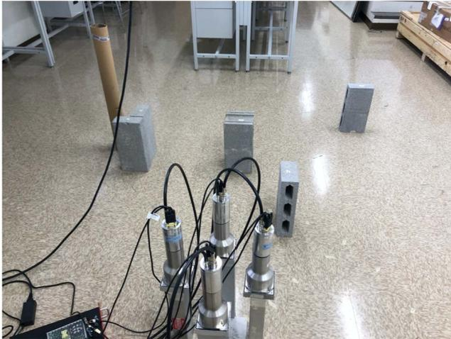
**Fig. 6.** Setup of L-Dataset 2 - This is a photograph of the detector array in the laboratory. The  $^{60}\text{Co}$  source is attached to the cardboard tube. The concrete blocks are the obstructions and cause the behavior of the gamma-rays produced by the  $^{60}\text{Co}$  source to be representative of an urban environment.
