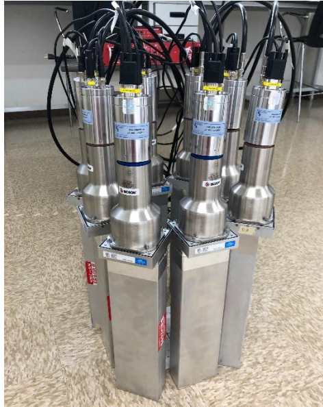
Figure 1. Detector array of eight NaI detectors in a cylindrical geometry.
