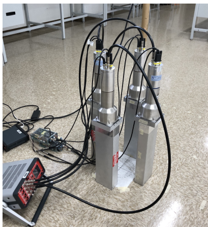
Fig. 2. Detector array and associated electronics. Source holder (brown) can be seen behind the array.
