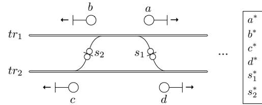
The segment consists of the two tracks ( $tr_1$  and  $tr_2$ ), two switches ( $s_1$  and  $s_2$ ) and four signal lights  $a-d$ . A switch is said to be in the *normal* state if it does not allow a train to switch tracks and in the *reverse* state if it does allow a train to switch tracks. If a signal is ON, it indicates that the train may proceed and if it is OFF, the train must stop. The direction of each signal is indicated by an arrow.
